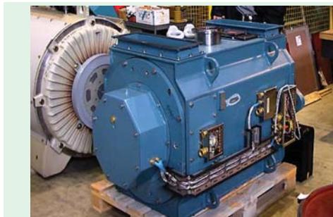
Induction motor for drilling applications
